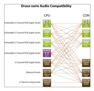
IHSE Draco KVM extenders now include comprehensive audio de-embedding and cross-conversion, reducing the number of modules required in a KVM system for audio handling and conversion in broadcast systems.
