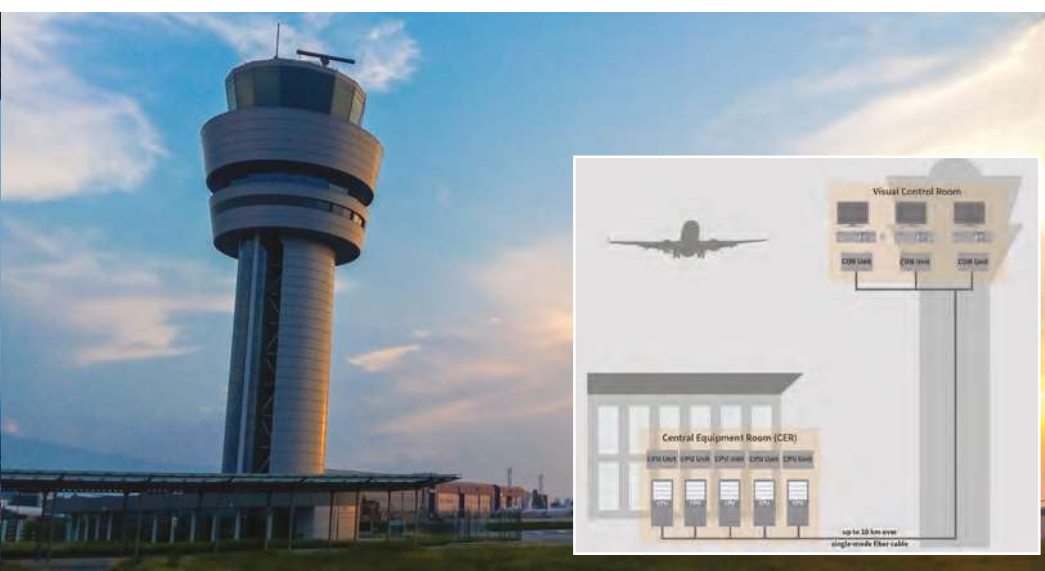
Above: KVM extenders connect controllers at the top of the tower to computers in the equipment room at ground level Inset: IHSE KVM technology transports real-time data throughout the entire air traffic control and management process, enhancing safety and operational efficiency from take-off to landing and beyond
