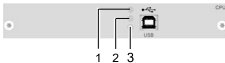
Fig. 2 Interface side add-on module USB-HID - Failure indication
