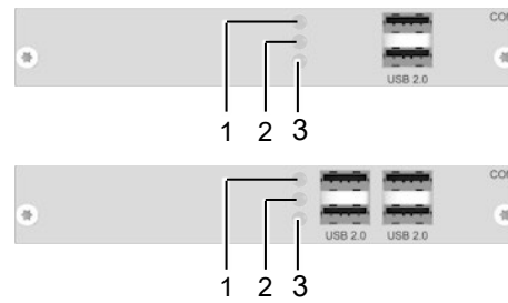
Fig. 3 Interface side add-on module USB 2.0 embedded - Failure indication
