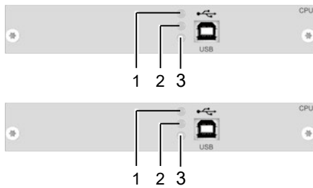
Fig. 3 Interface side add-on module USB 2.0 embedded - Failure indication
