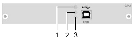
Fig. 66 Interface side add-on module USB-HID - Status LEDs
