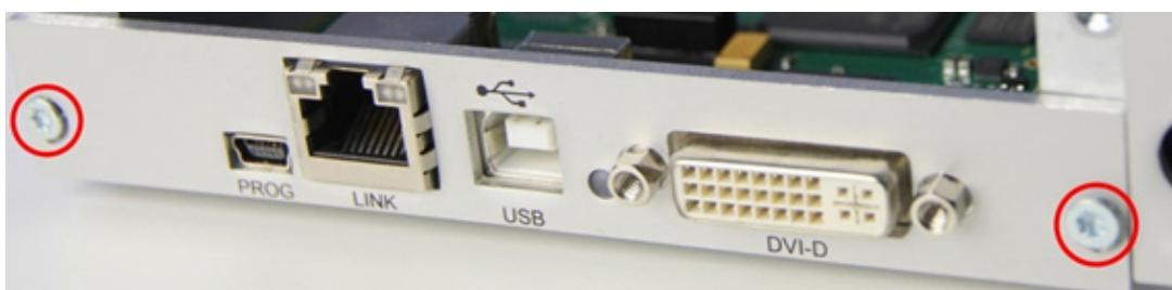
Fig. 48 Front view - Front panel with fastening screws
