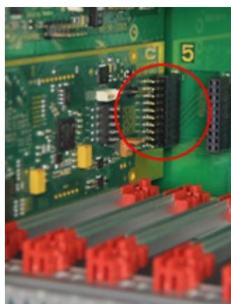
Fig. 66 Add-on module mounted in a 21-Slot slide-in chassis
