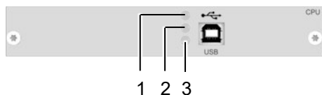
Fig. 50 Interface side add-on module USB HID - Failure indication
