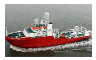
The 65 meter MV Fugro Searcher is a new, highly equipped geophysical survey vessel providing an acoustically quiet and stable platform for operation in the North Sea and International waters. The vessel is equipped with an array of echo sounders, sonar equipment and sea-bed profilers to service the offshore oil and gas and cable engineering industries.
