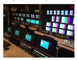
At each workstation terminal the operator has full instantaneous interactive control of the host PC including USB HID, USB 2.0 connection. RS232 controls and audio feeds are also accommodated providing greater flexibility and ensuring that all features are included in the overall system.
